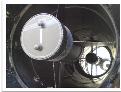
Figure 17: Sketch of a telescope (left) - incoming flux density  $F$  in  $\text{W/m}^2$ , surface area  $A$  in  $\text{m}^2$ . The area covered by the sensor (or often a secondary mirror) is called the obstruction. The right photograph shows the view into the tube of ESA's OGS telescope, giving an impression of the central obstruction.
